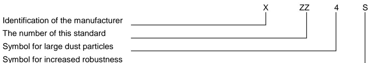
In place of symbols 3 and 4 in the above examples the symbols 5, 8 and 9 would be used to indicate frames for protection against gases and fine dusts (5), short circuit electric arc (8) and molten metals and hot solids (9).
