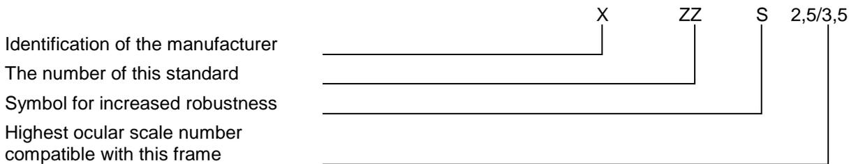
This marking would be applied to a goggle or faceshield frame intended for use with UV filter(s) (with or without good colour recognition) up to a scale number of 2.5 or 3.5
