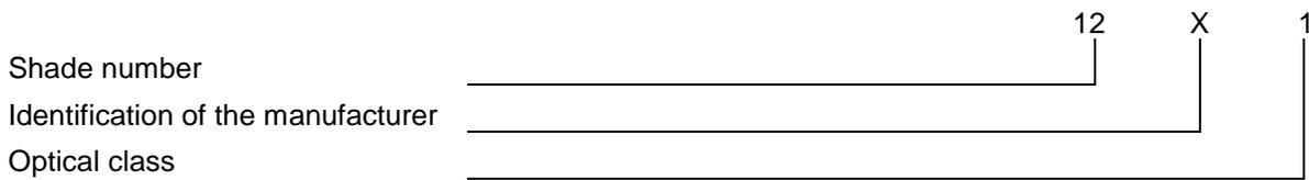
b) welding filter with mechanical strength function
