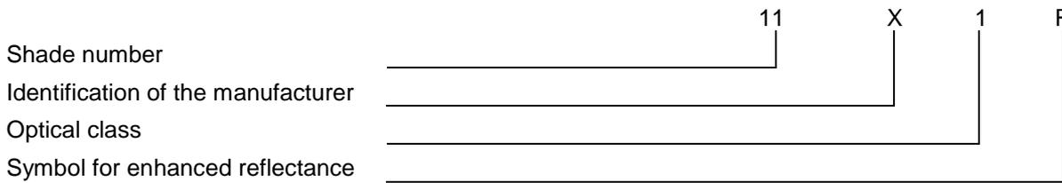
For marking photochromic sunglare filters, the scale numbers corresponding to light and dark shall be separated by the symbol < for example 5 - 1,4< 2,5 X 1.
