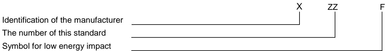
In place of the symbol F in the above example the symbol B would be used in the marking of a frame used for protection against high speed particles of medium energy impact, and the symbol A in the marking of a frame used for protection against high speed particles of high energy impact. Additionally, if the frame was for use against high-speed particles at extremes of temperature the impact symbols would be followed by the letter T; i.e. FT, BT or AT.
